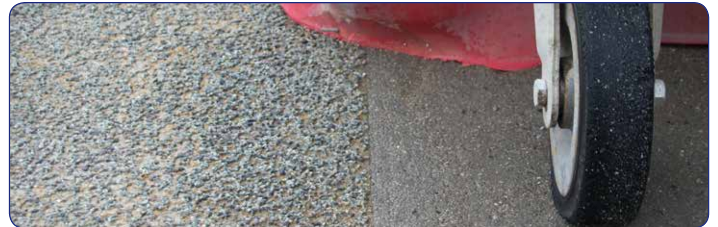
Wide-area cleaner: Improving roughness by using high-pressure water
